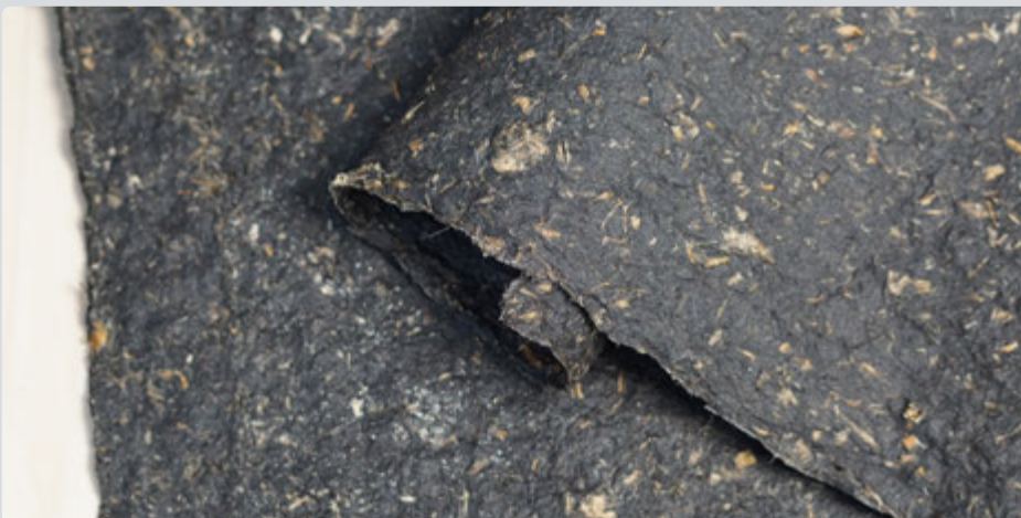
IMAGE 5. Water hyacinth pulp mixed with binders to make leather. (3 March 2023, Barcelona- Spain, Nanditha Nair, Copyright of Nanditha)
