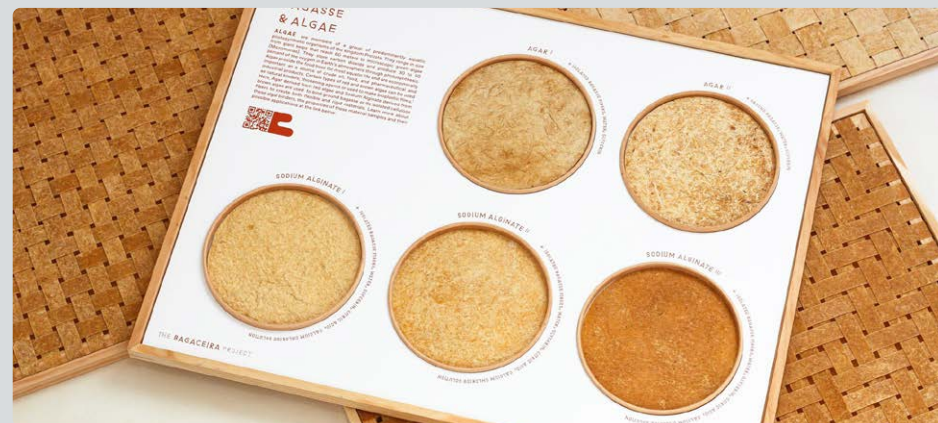
IMAGE 2. One of the eight Bagaceira material library display cases. This case displays 5 samples made with algal binders (Barcelona, 2023, Julia Steketee)
