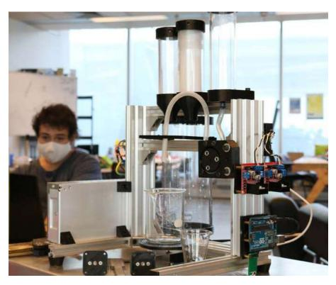
Second Iteration of the Biomixer, assembled with durable and market-available materials like standard aluminum profiles, acrylic tubes and machined parts, projecting its replication. (2020, Santiago de Chile, Fab Lab U. de Chile + students)
