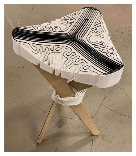
Parameterization of 3D printable furniture using generative design.
