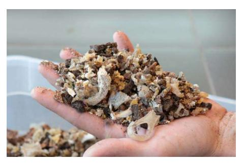
Grinded Agar agar based biopolymers and other biomaterials mixed with organic waste to analyze how these biobased materials react to compost in a certain period of time. (2020, Santiago de Chile, Fab Lab U. de Chile)
