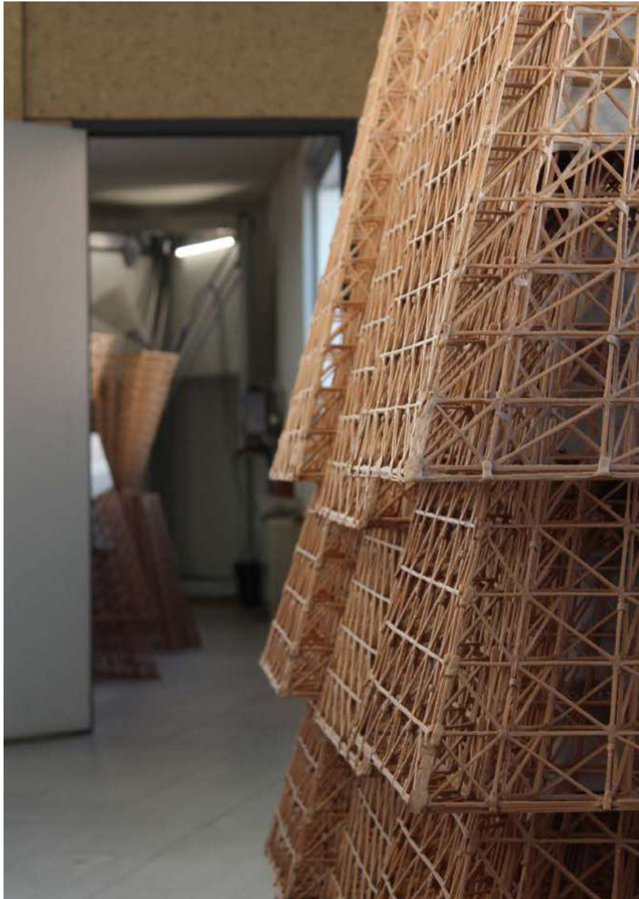
3D printed modules for Conifera, the architectural installation designed by arch. Mamou Mani for COS at the Fuorisalone Milano 2019, that came to life thanks to the power of the network: four hubs that shared knowledge and machines helped realize and craft the over 700 pieces. 2019, ©Fab Lab Venezia
