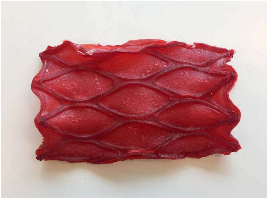
Researching assembly modes with same molds but progressive variations of the biopolymer formula (2019, Santiago de Chile, Fab Lab U. de Chile + students Macarena Inostroza and Dominique Barros)
