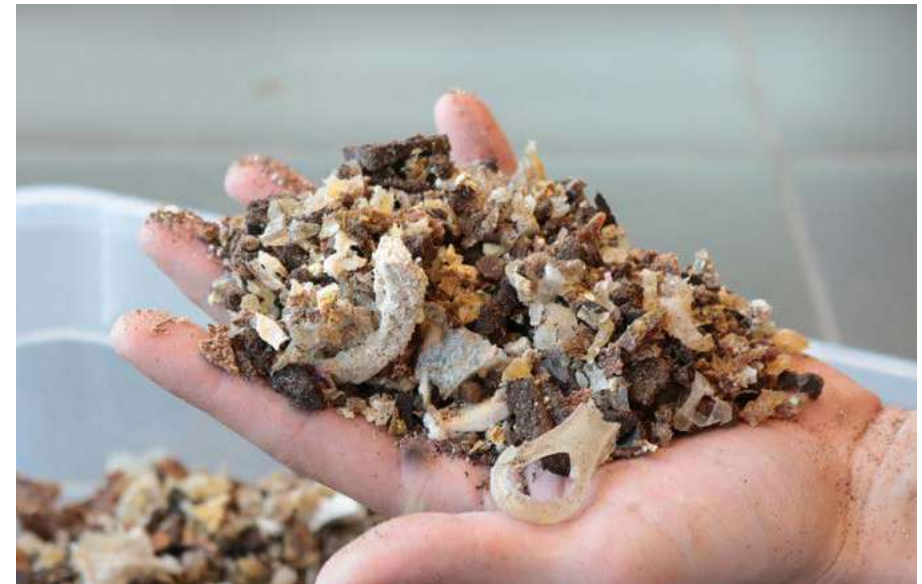
Grinded Agar agar based biopolymers and other biomaterials mixed with organic waste to analyze how these biobased materials react to compost in a certain period of time. (2020, Santiago de Chile, Fab Lab U. de Chile)
